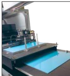
*Change from pano to broadsheets in a matter of seconds with the Quickswitch module.*
